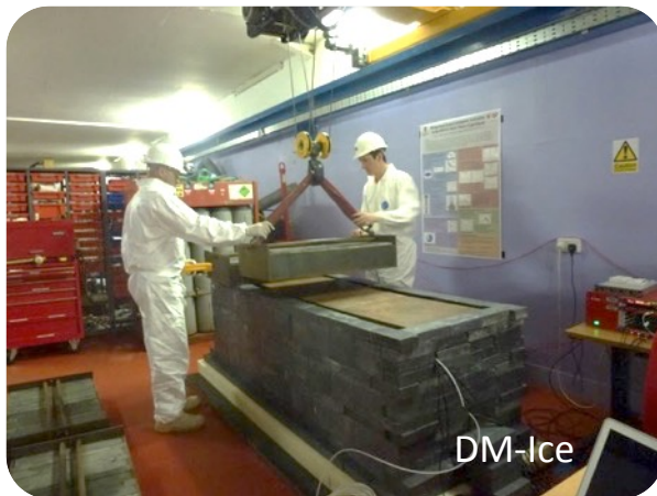
DM-Ice: 250kg NaI(Tl) array for studying WIMP annual modulation
