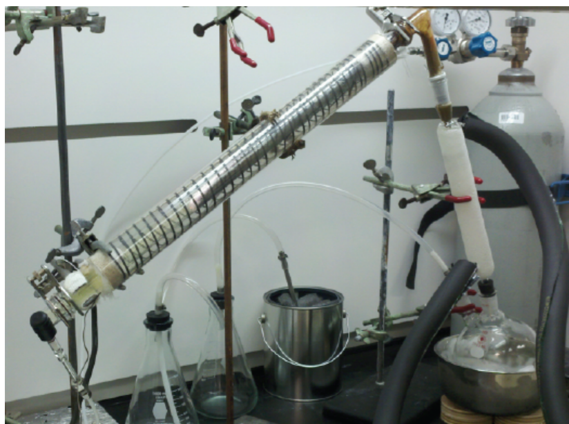
Ge reduced in Chlorine gas
