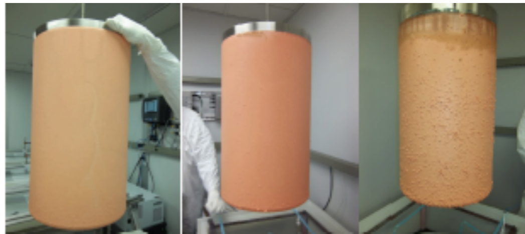
Inspection of EF copper on mandrels
