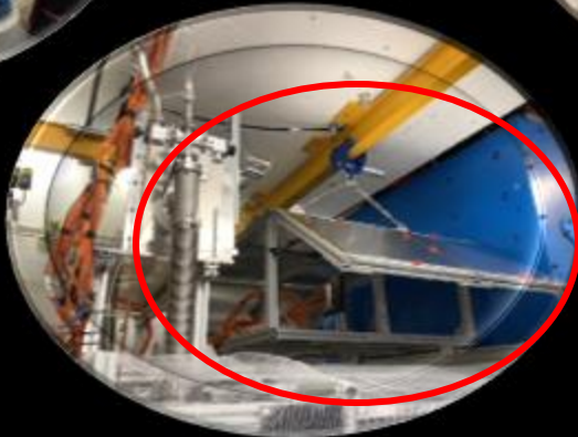
VELO-TOP NTD array installed
