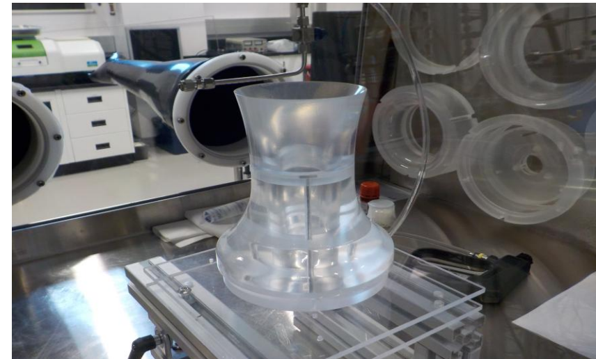
Coated piece ready to be sealed and shipped to Sudbury
