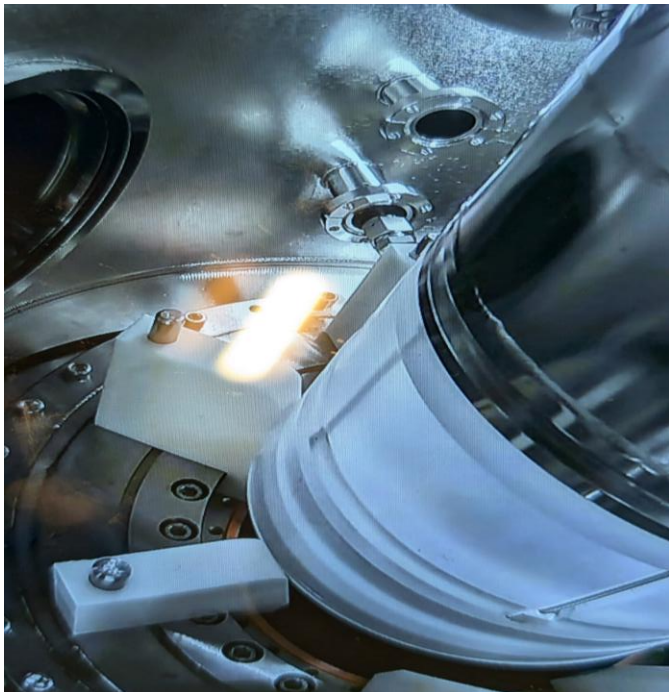
Flowguides and neck installed in the glovebox and being lowered into the detector
