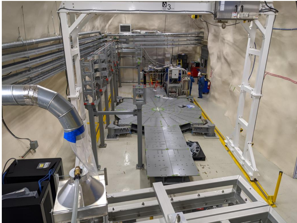
March 2023 Dilution fridge underground for stand-alone testing
