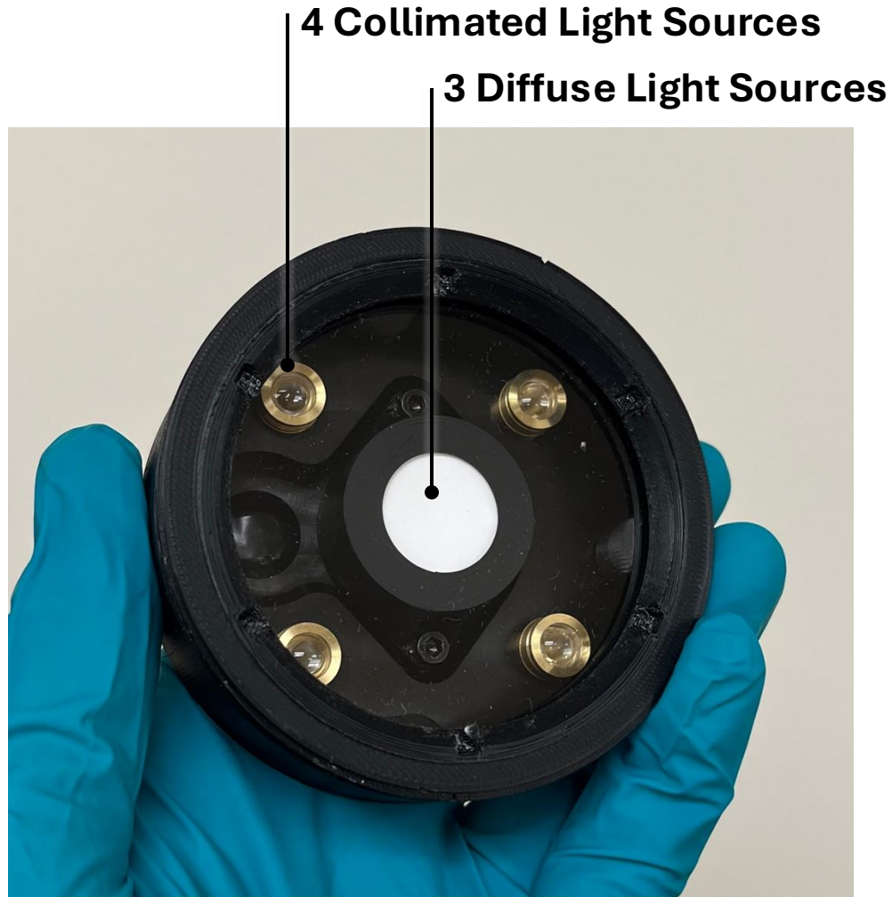
LED System with Latest Diffuser Design
