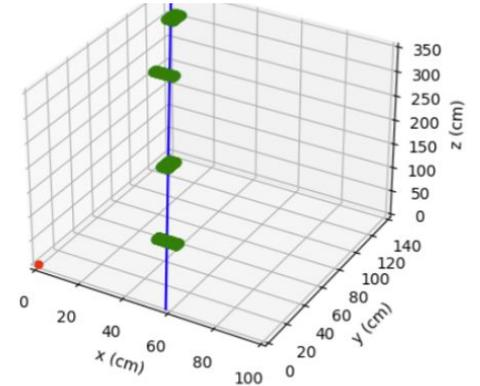
Cosmic ray events in the UVic MATHUSLA prototype, and a reconstructed muon track passing through all four layers
