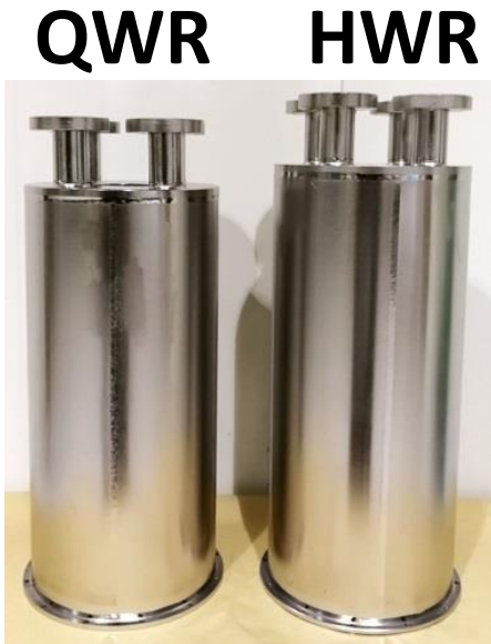
QWR: Quarter Wave Resonator HWR: Half Wave Resonator
