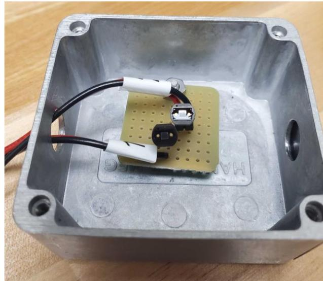
2 SiPMs (in box) connected to Citiroc, cooled down to 10°C
