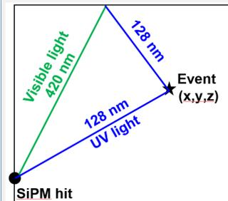
Time-of-flight corrected SiPM residual time
