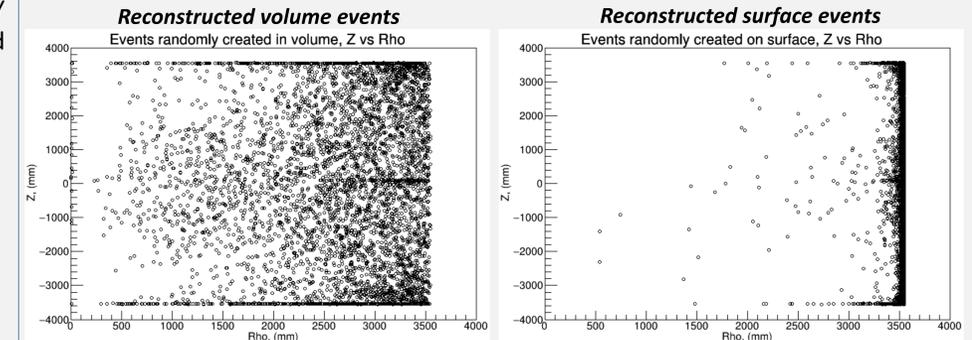
The time fitter needs some improvement due to observed misconstructions. Specifically, there are fewer events reconstructed in the middle of the detector compared to the surface, despite the events being uniformly created throughout the volume. Additionally, there are extra events reconstructed at the center while the events being created on the surface, indicating inaccuracies in the time fit.
