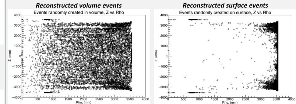
The charge fitter demonstrates reasonable reconstruction accuracy for events uniformly distributed within the volume, as opposed to the time fitter. However, there is a small area where no events are reconstructed. The charge fitter's performance is less optimal in reconstructing surface events compared to the time fitter. Specifically, fewer events are reconstructed at the top and bottom of the detector compared to the barrel surface, despite the uniform creation of events across the surface.
