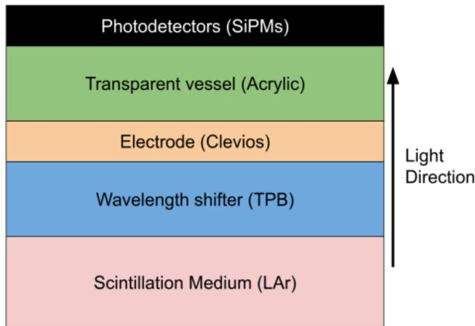
Order of coatings on the acrylic vessel for DarkSide-20k. Layers not to scale.
