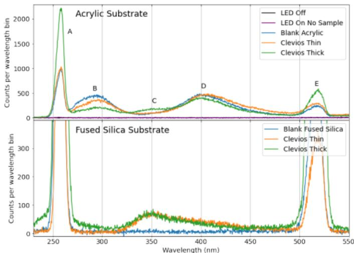
Emissions spectra for Clevios on acrylic substrates (top) and fused silica substrates (bottom)
