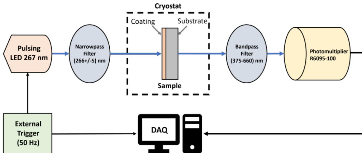
Schematic diagram of the apparatus used to take time-resolved measurements
