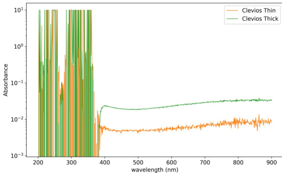
absorbance measurements from samples with acrylic substrates.
