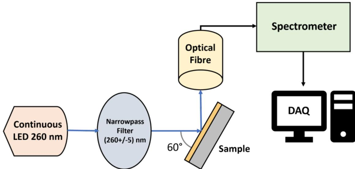
Schematic diagram of the apparatus used to take same side emission spectra.
