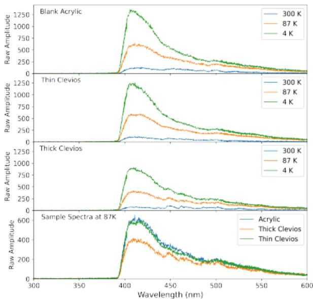
Emission spectra for blank acrylic, thick Clevios, and thin Clevios at 300K, 87K and 4K.
