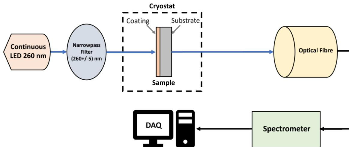
Schematic diagram of the apparatus used for emission spectra.
