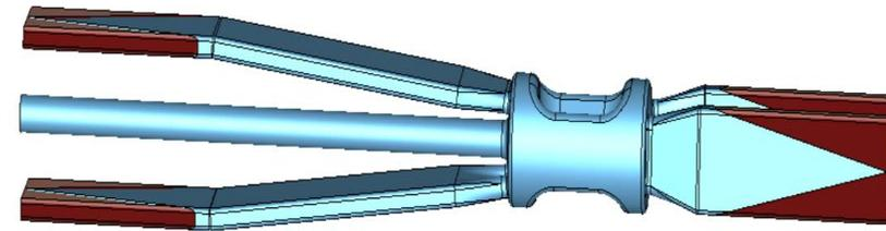
394 MHz Crab Cavity with waveguide HOM extraction to damped loads
