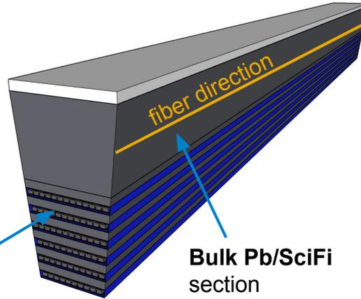
4(+2) layers of AstroPix interleaved with 5 Pb/SciFi layers
