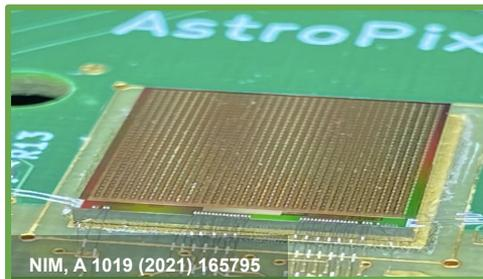
Insert layers of monolithic **AstroPix** silicon sensors (ultra-low-power, developed for NASA at ANL) to capture a **3D image of the shower**
