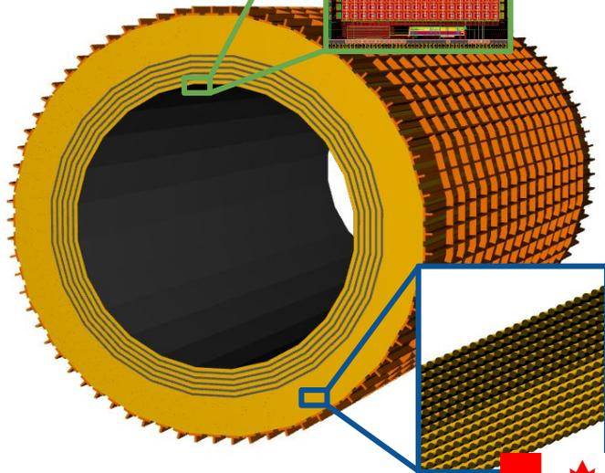
**Pb/Scintillating fiber** layers with two-sided SiPM readout
