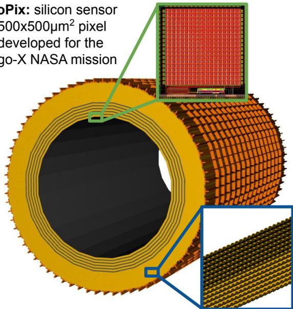
**Pb/Scintillating fiber** layers with two-sided SiPM readout
