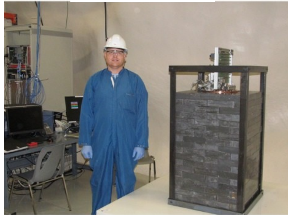
Lead shielding at appropriate thickness
