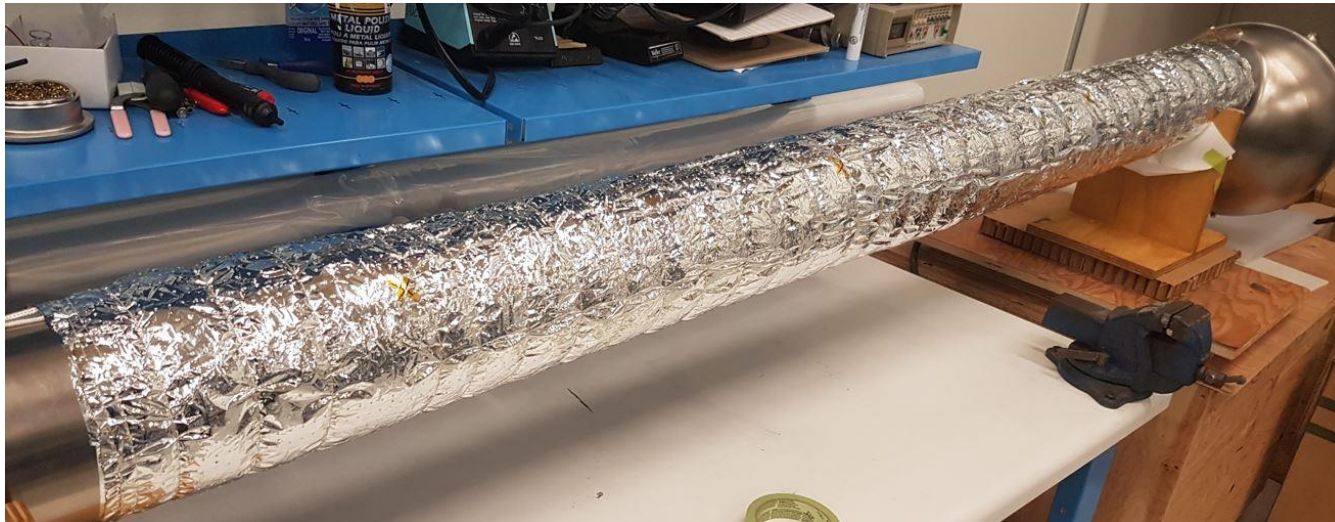
“Wall 1” in kapton super-insulation, all sensors installed
