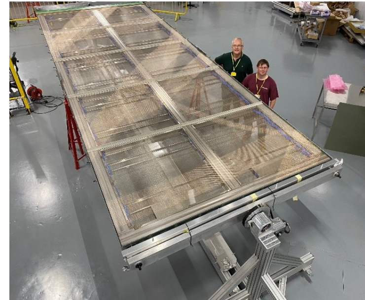
APAs being tested at Daresbury Laboratory, UK; one 2.3m x 6.3m APA is shown
