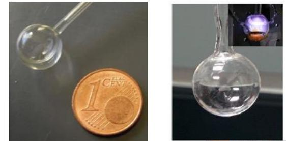
Absolute probes all cross-calibrated at ANL test magnet
