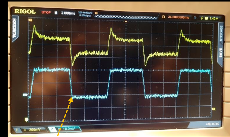
Switching of B field at MOT position in < 1ms.
