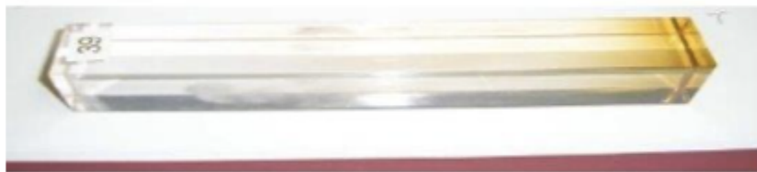
Example of damaged block from radiation (DVCS experiment)
