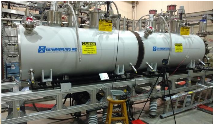
Electron beam ion source EBIS with polarized ^3\text{He} extension
