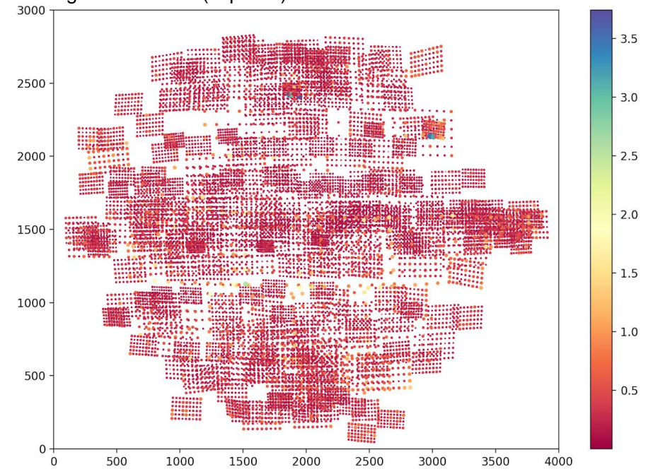
Reprojection errors for "clear" images as a function of image coordinates (in pixels).
