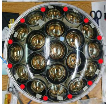
Continuous LEDs in mPMT module provide photogrammetry targets.
