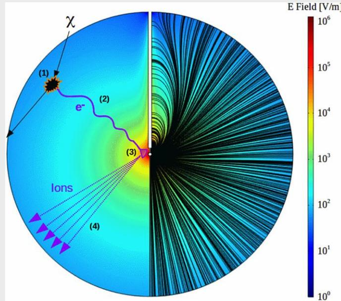
WIMP detection principle (left) and electric field inside an SPC (right)
