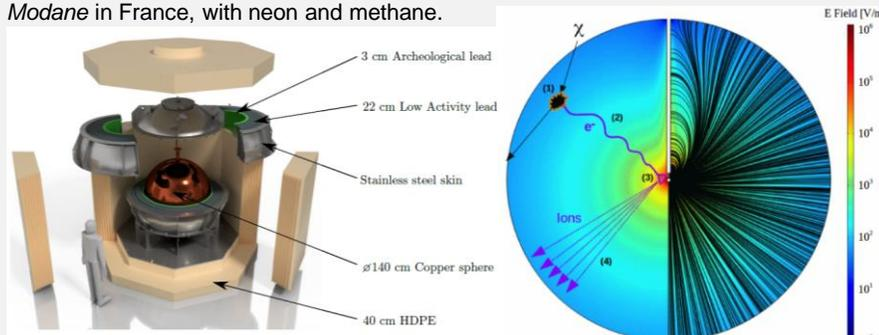
Figure 1 a) Schema of the outside shielding b) Detection mechanism
