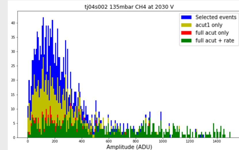
The saturated alpha signals can be broken up and difficult to detect, but using the drift time, rate of events and decreasing baselines, we can identify alphas and remove most of the low-energy background due to them with a 5s cut after each alpha, keeping 85-90% of the total time.
