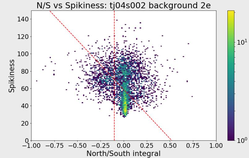
A cut on N/S removes fat pulses (dominant in 2-peak data) and a Fisher discrimin. cut removes spikes.
