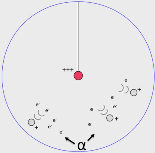
There is  $^{210}\text{Po}$  contamination in the copper surface, which causes alphas that ionize a lot of gas. All the ions create a space charge that disturbs the electric field, and changes the electron drift time. For some still unknown reason, a high rate of low energy events keep happening for around 5s after each alpha.
