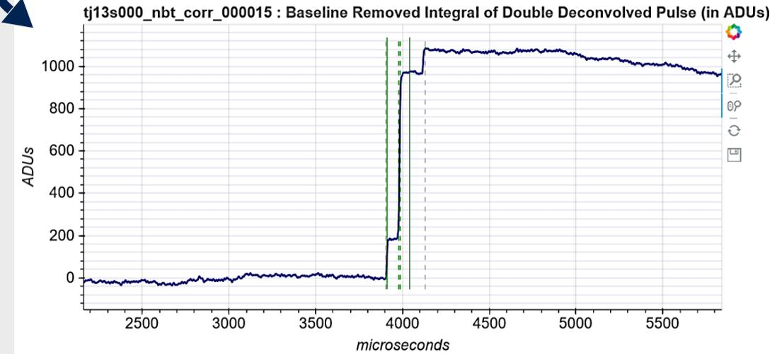
The ballistic deficit is the signal amplitude that gets underestimated due to the exponential decay of the preamplifier. The full amplitude (energy) is retrieved by doing a double deconvolution of the raw signal, and then integrating the pulses.
