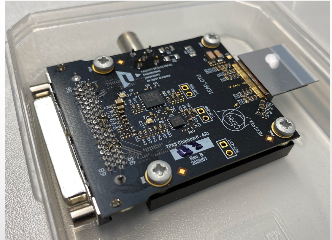
Timepix-3 detector for Run-3
