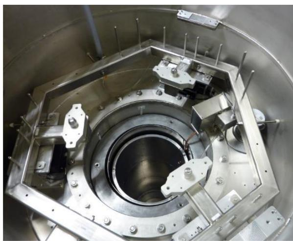
CUTE drywell: suspension system and shielding
