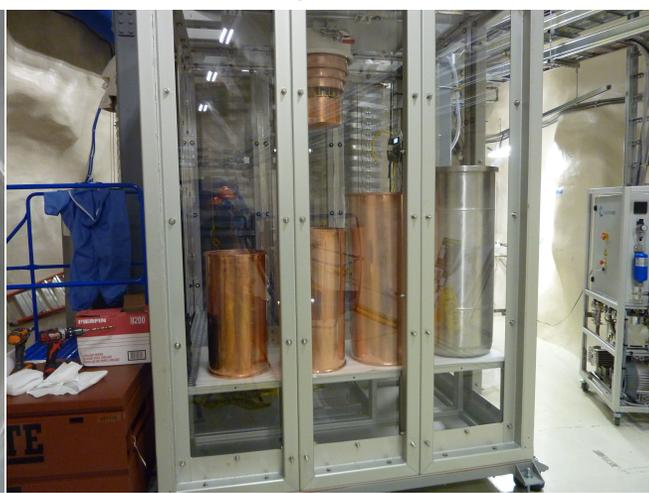
CUTE cryostat open inside the CUTE cleanroom layers
