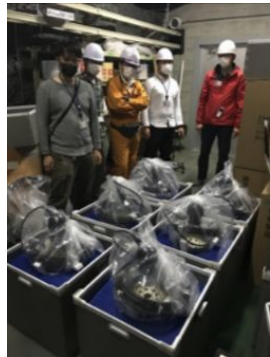
HK PMTs were checked according to the pre-calibration manual to install HK PMTs in 2018 for SK.
