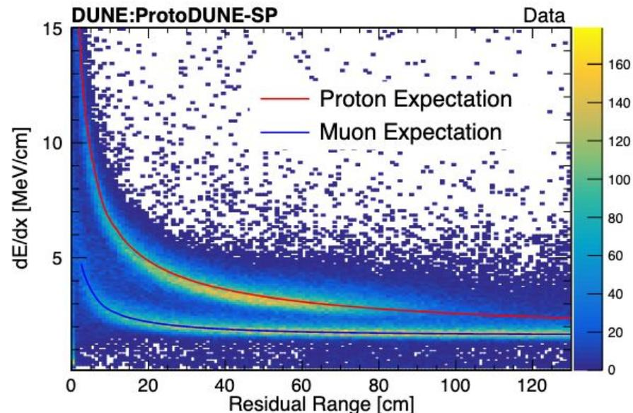
Detector response calibration based on cosmic muons
