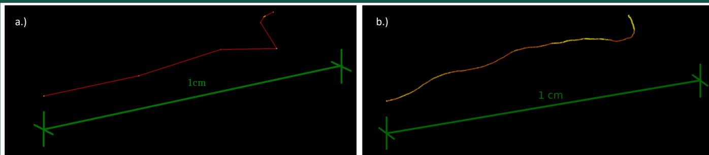
Fig. 4 a.) Multiple scattering and b.) Single scattering 2 MeV electron trajectory
