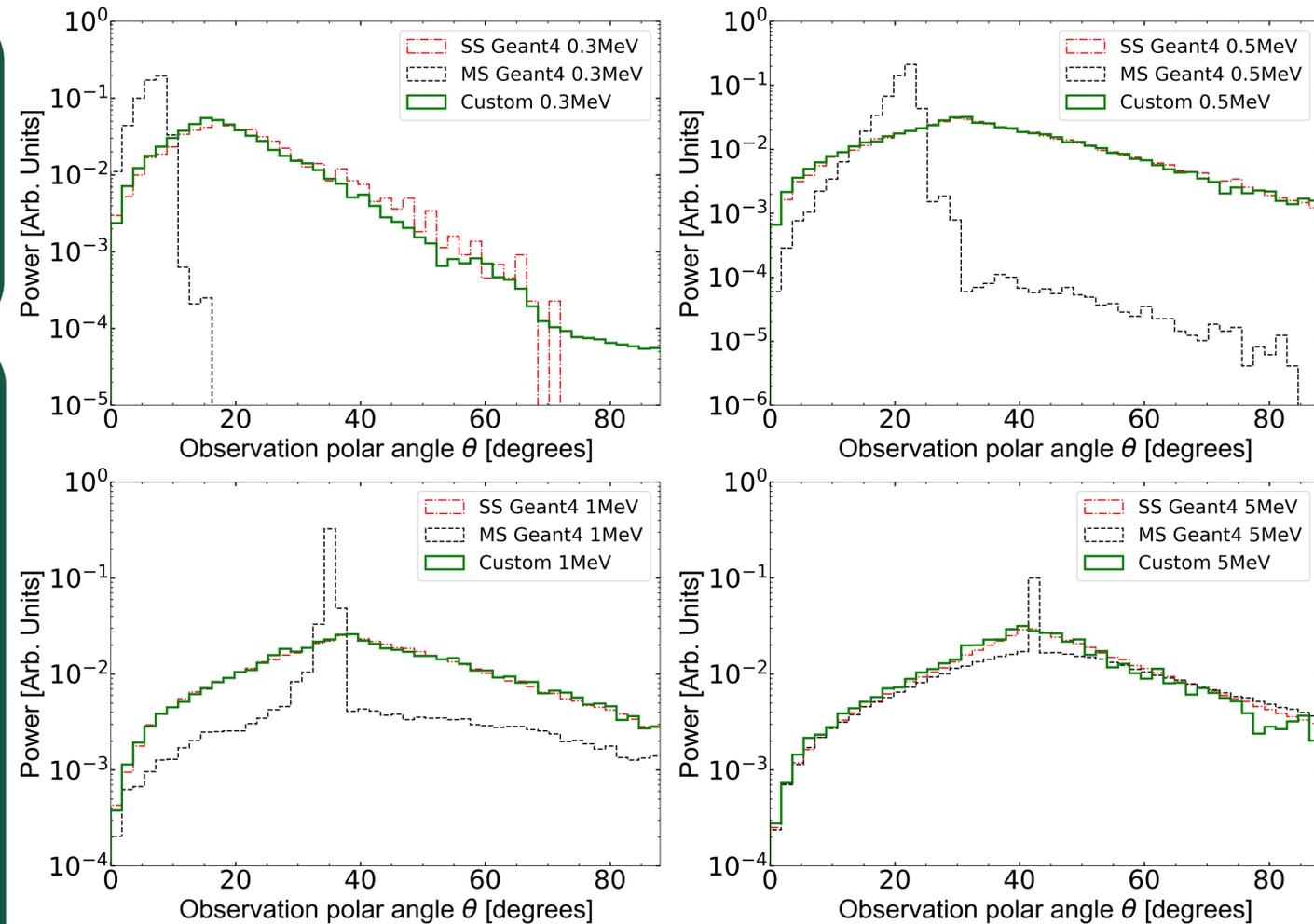
Fig. 3 Angular dependence of the Cherenkov light as they would be observed in a spherical detector, created by the electrons injected along the z-axis. SS – single scattering, MS – multiple scattering.
