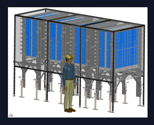
Active scintillation counter detector with a large path length of sensitive scintillator bars.
