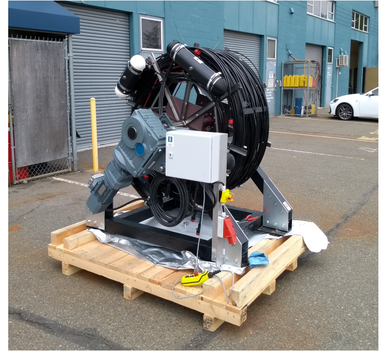
One of the two STRAW strings spooled onto the deployment winch
