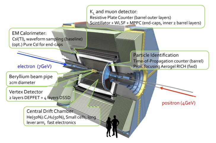
Reusing solenoid, iron, part of muon system, calorimeter crystals. Remainder optimized for rates and high backgrounds
