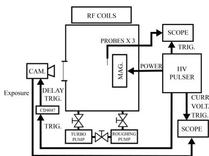
Figure 2: Experimental setup diagram.
