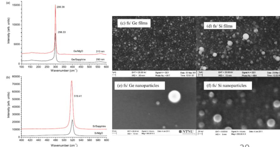
Fig. 8. Raman spectra of fs laser deposited (a) Ge and (b) Si films.
