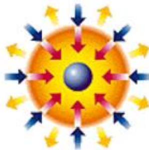
2) Compression: Fuel is compressed by the rocket-like blowoff of the hot surface material.
