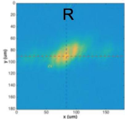
XUV pulse focused on target by an ellipsoidal mirror
