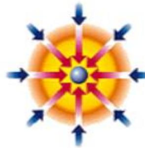
3) Ignition: During the final part of the laser pulse, the fuel core reaches 20 times the density of lead and ignites at 100,000,000 degrees Celsius.
