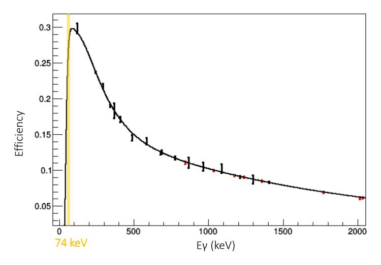
$\epsilon_{\gamma}$  changes quickly at low energies, so a well-calibrated efficiency curve is crucial
