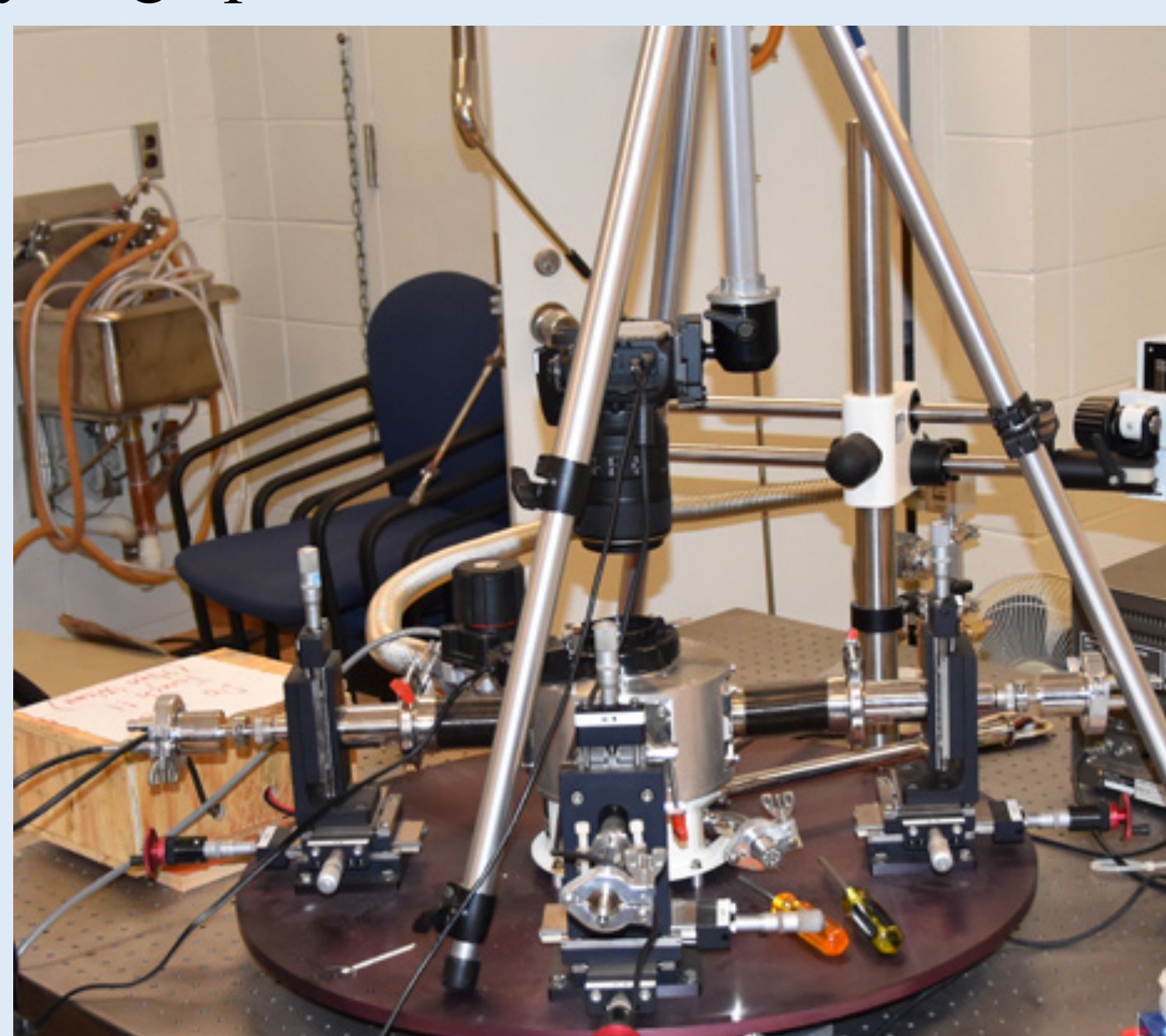
Figure 2: A Janis ST-500 micromanipulated probe station.
