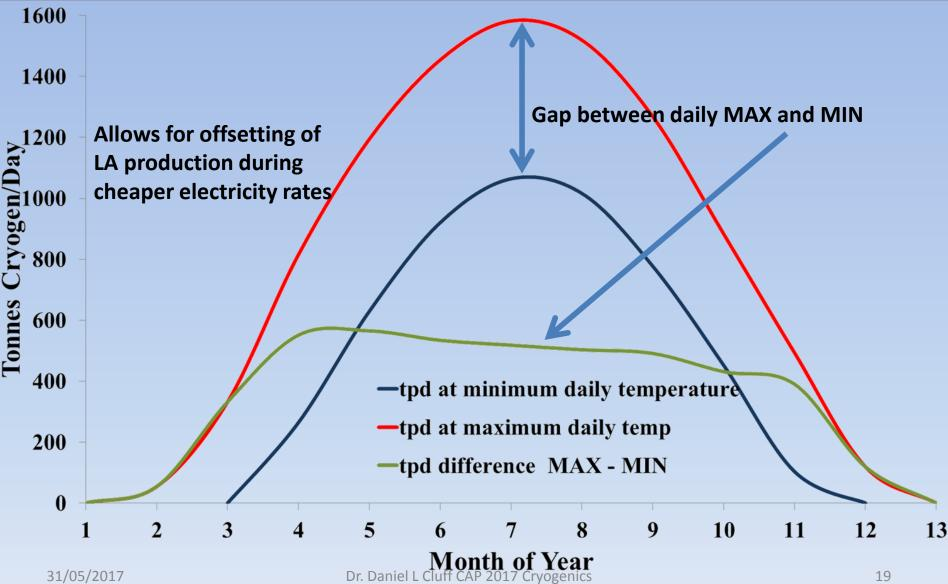
Cryogenic Chilling for Actual Temperature Fluctuations 07/07/2010 One of the hottest days in 2010
