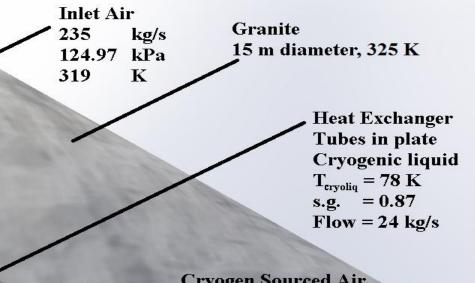
Cryogen Sourced Air Perpendicular to Shaft Air Flow T<sub>cryoga</sub>,78 to 85 K on Exit Density about 4 kg/m
