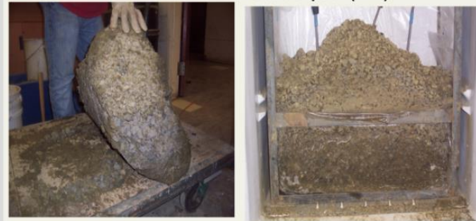
Sept 26/08 (60% rockfill/40% tailings) 6% - 7% water
