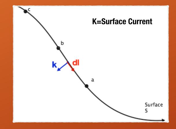
If the contours are equally spaced then the surface current is the same between each of the contours and can be approximated by equally spaced wires in contours of constant  $\Delta U$
