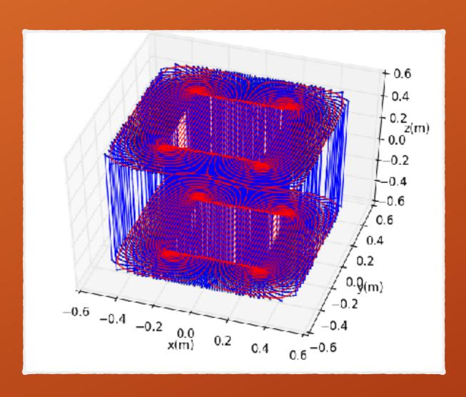
Main coil=64 turn End cap=4 turn Right: Main coil=256 turn End cap=32 turn
