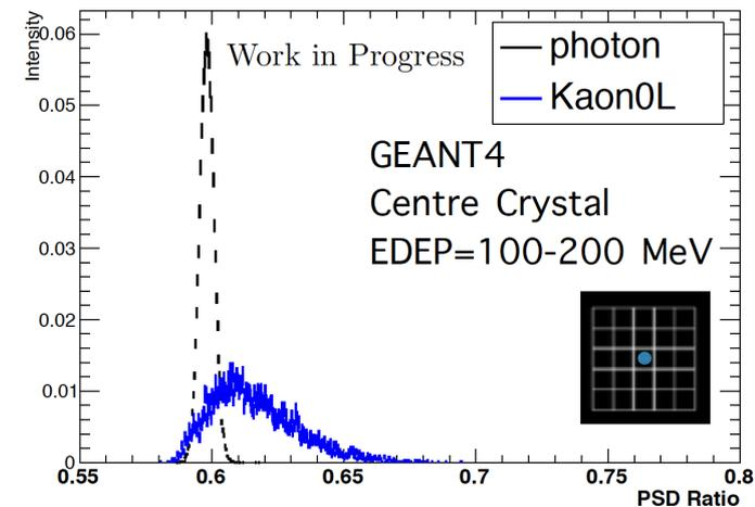
Simulation of photon and  $K_L$  pulse shapes
