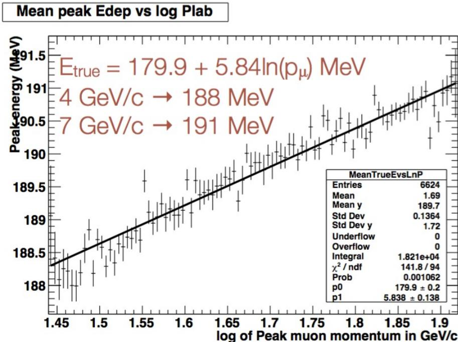
Sub-1% calibration of barrel crystals possible in Phase 2 with  $\sim 4\text{fb}^{-1}$  of data
