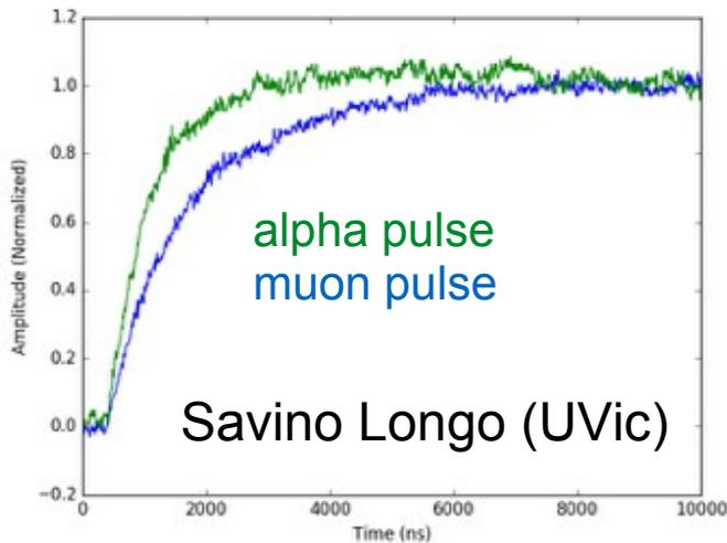
Characterize pulses with ratio of charge at  $t=1.2 \mu\text{s}$  and  $t=7.4 \mu\text{s}$
