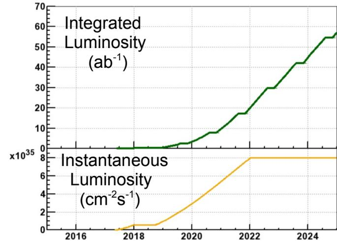
Luminosity to  $\sim 8 \times 10^{35}$  by 2022 with ultimate target of  $50 \text{ ab}^{-1}$  recorded
