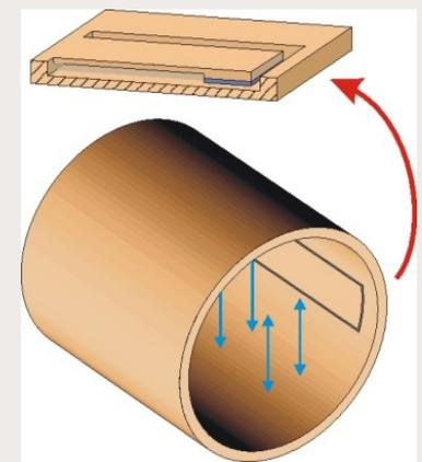
Resonator Prototype at SFU ( $Q \sim 300$ )
