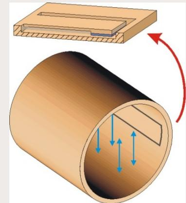
Resonator Prototype at SFU (Q ~ 300)
