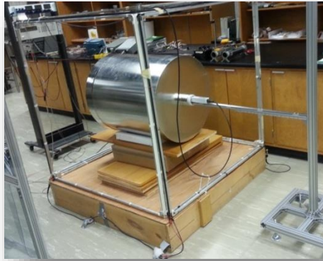
Cylindrical shells of the 4 layer FM shield
