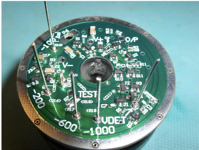
Preamplifier with HV divider
