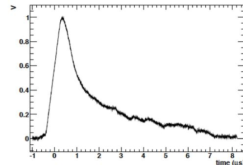
He-3 detector signal of thermal neutrons from UVic neutron source
