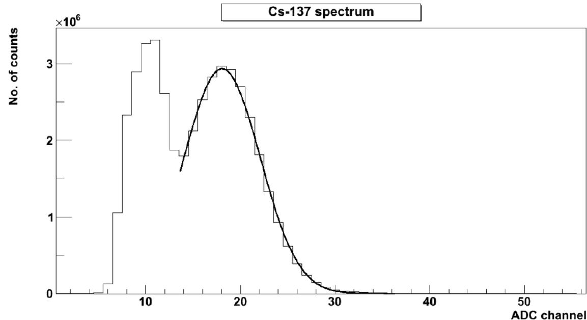
$^{137}\text{Cs}$  spectrum measured with a pure CsI crystal, photopentode, and Montreal preamplifier
