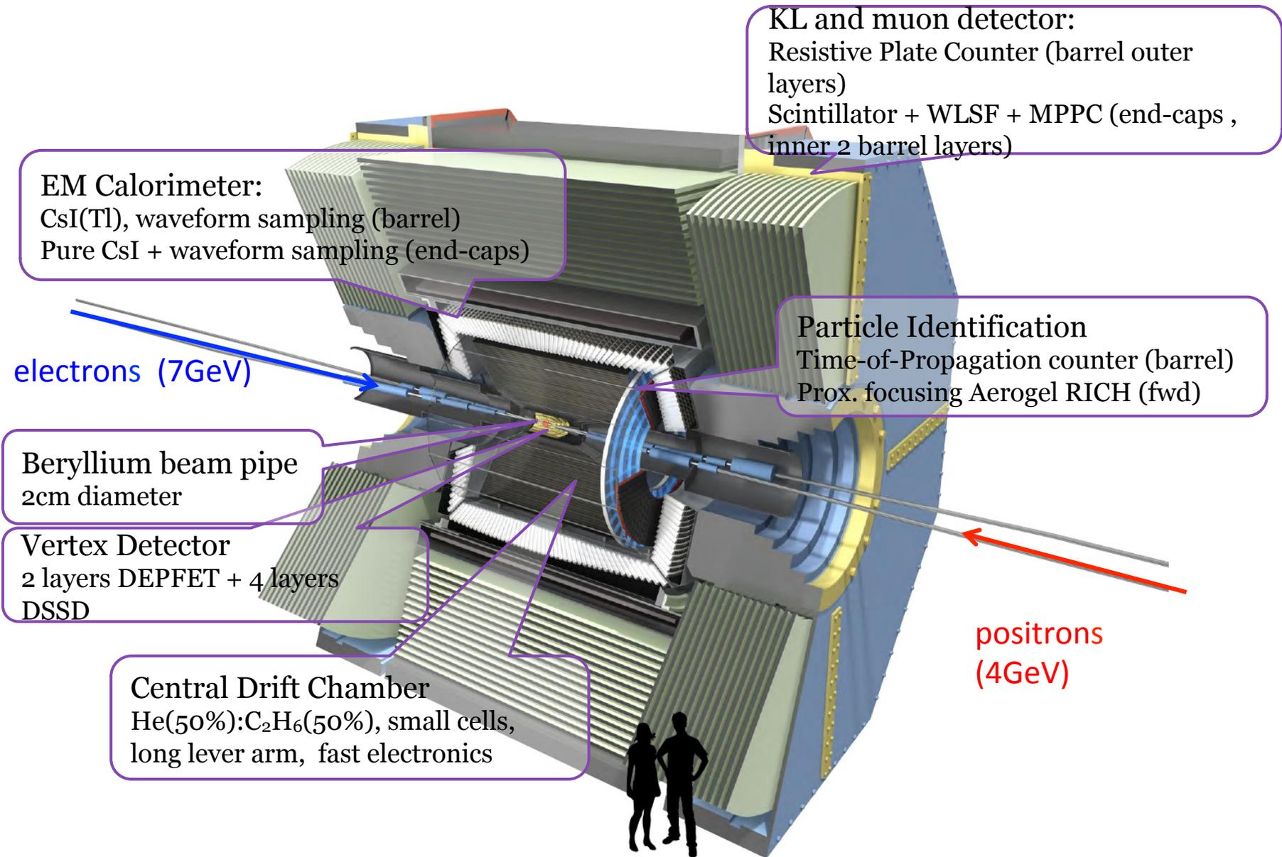
EM calorimeter: upgrade needed because of higher rates barrel: waveform sampling electronics
