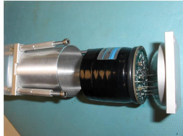
Photomultiplier mounted with preamplifier and Faraday cage
