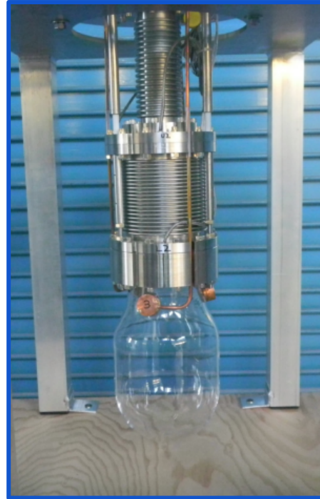
PICO-2L 2-bellow design inner vessel assembly
