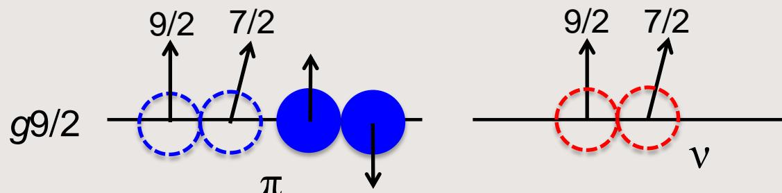
Interaction between pairs of pn hole pairs lowers the  $16^+$  state below the  $12^+$
