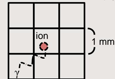
Measure  $\gamma$ -rays of isomer after implantation
