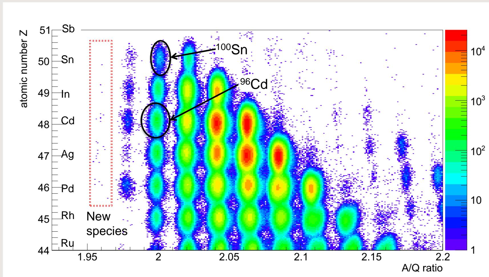
2317  $^{100}\text{Sn}$  ions, ~18000  $^{96}\text{Cd}$  ions produced and identified
