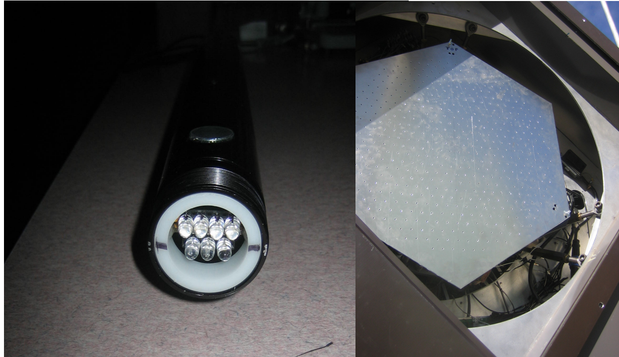
UV-LED Calibration System
