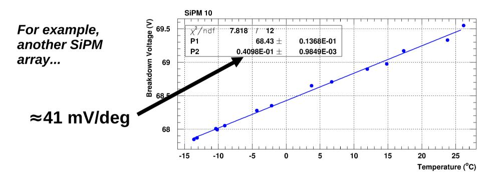
Without evaluation of each individual SiPM array, the 10%-accurate operation is possible in the temperature range of few degrees only.
