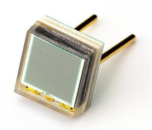
Matrix of avalanche photodiodes (APDs) built on the same Si substrate
