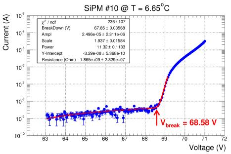
Measurements were done with Keithley 6471 picoammeter/voltage source
