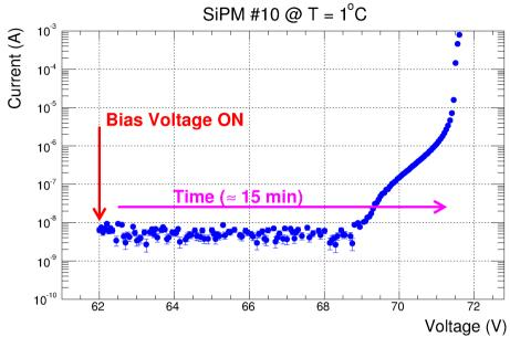
Measurements should be started only after 30-45 minutes of SiPM "warming"
