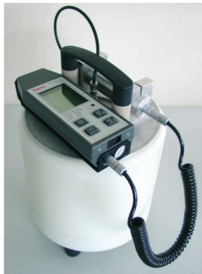
FHT 762 Wendi-2 Neutron Detector, by Thermo-Fisher.
