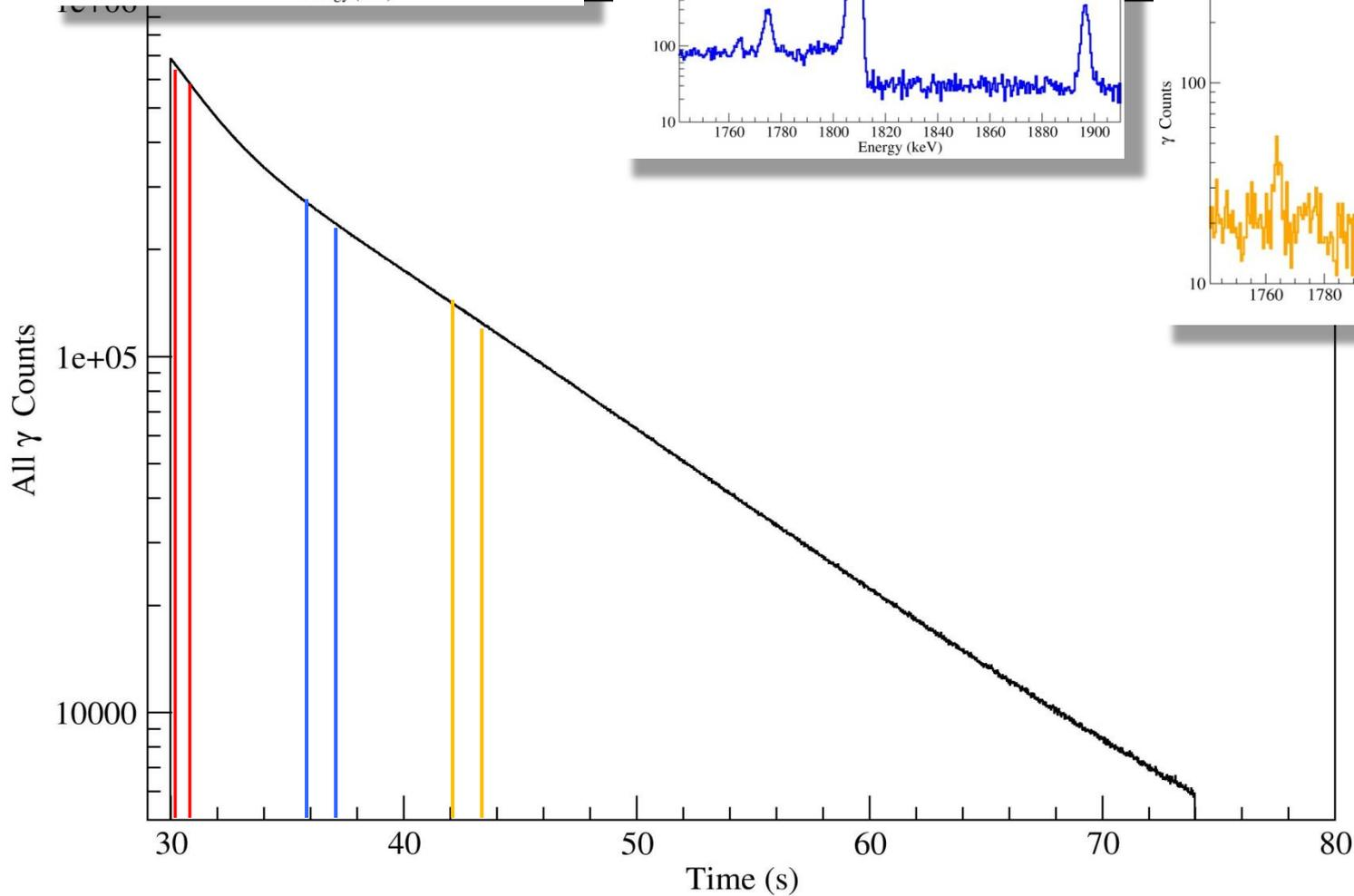
Fit 1809 keV peak area vs. time with  $^{26}\text{Na}$  and  $^{26}\text{Al}^m$  components
