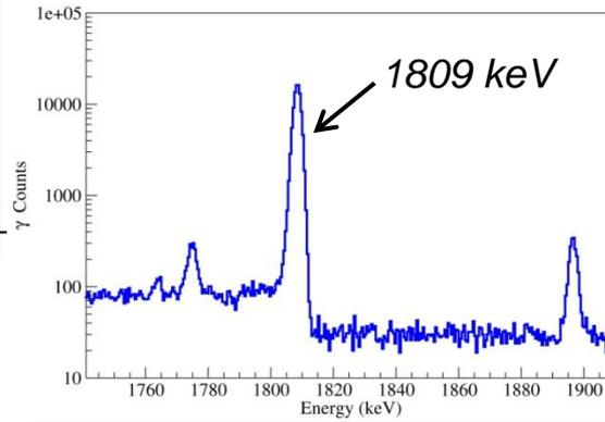
Fit 1809 keV peak area vs. time with  $^{26}\text{Na}$  and  $^{26}\text{Al}^m$  components
