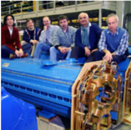
LHC deaning insertion quadrupoles produced in Canada (Copyright TRIUMF)
