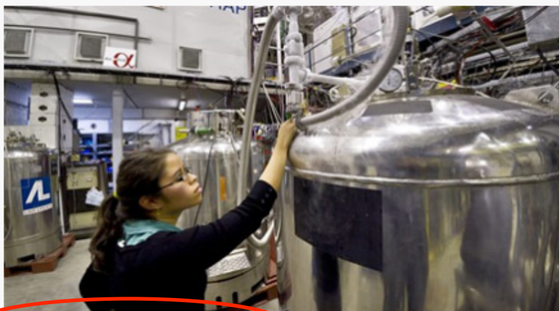
Andrea Gutierrez, a PhD student from UBC, transfers liquid helium from a storage dewar into the cryostat containing the superconducting magnetic trap used by the ALPHA experiment.
