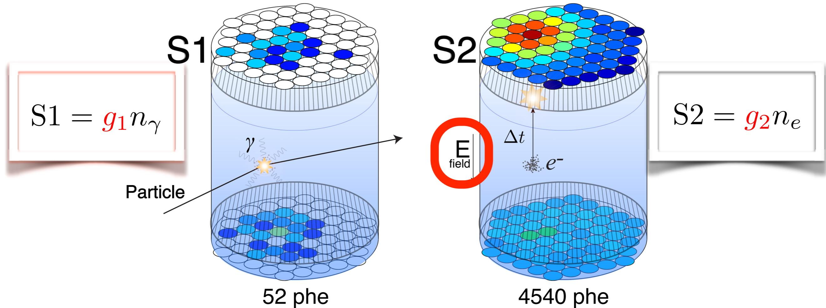
$g_1$ ,  $g_2$  and **drift field** are the crucial parameters
